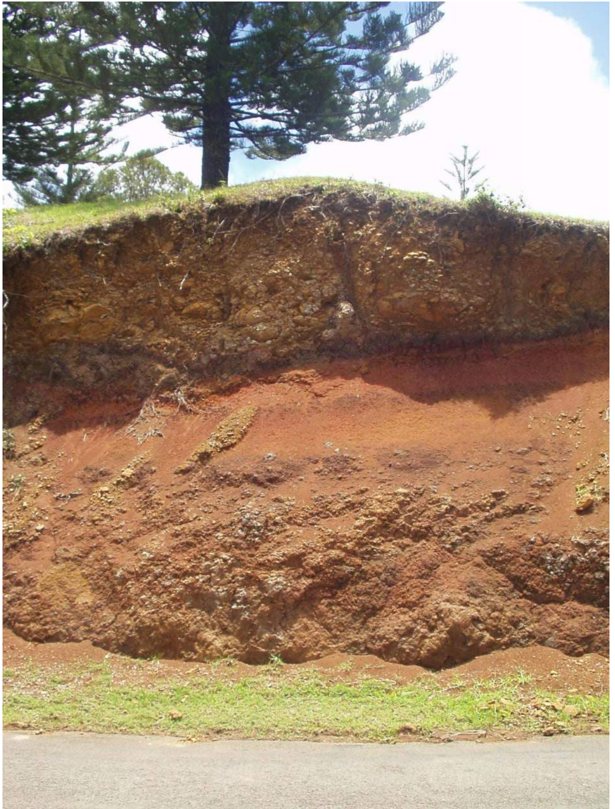
Plate 1: Basalt flow overlying a residual soil formed by a previous basalt flow.
