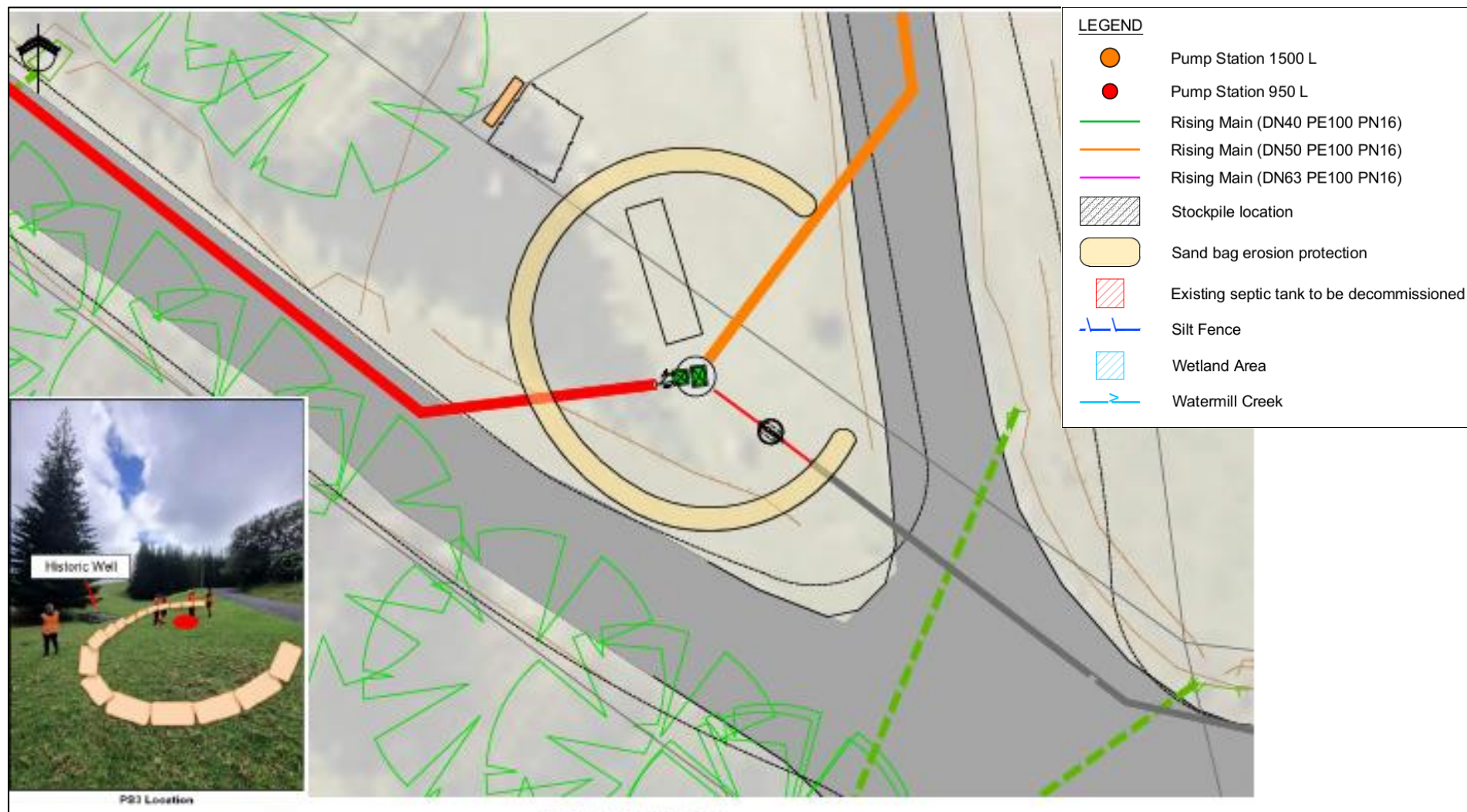
Figure 7.2-6: Erosion and Sediment Control Plan (indicative) - PS3 site
