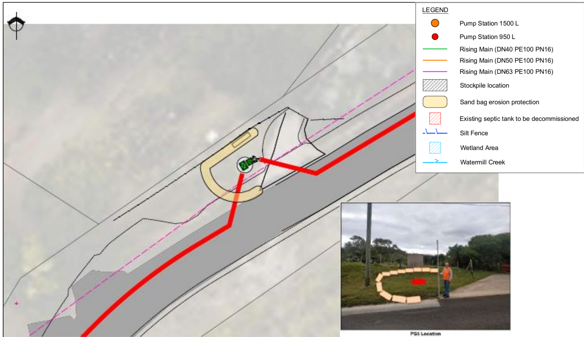
Figure 7.2-8: Erosion and Sediment Control Plan (indicative) – PS5 site
